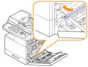
3 Carefully remove the misfed paper in the direction shown.
